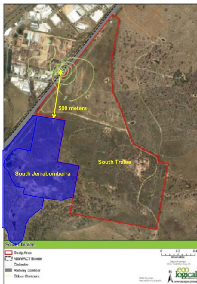
Figure 7-1: Predicted odour concentrations at the 99th percentile due to the asphalt plant stack
